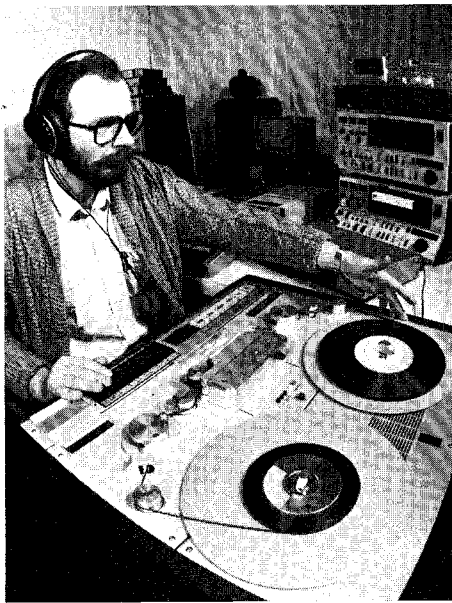
A Studer A820 transfers the incoming mastertapes to PCM.
