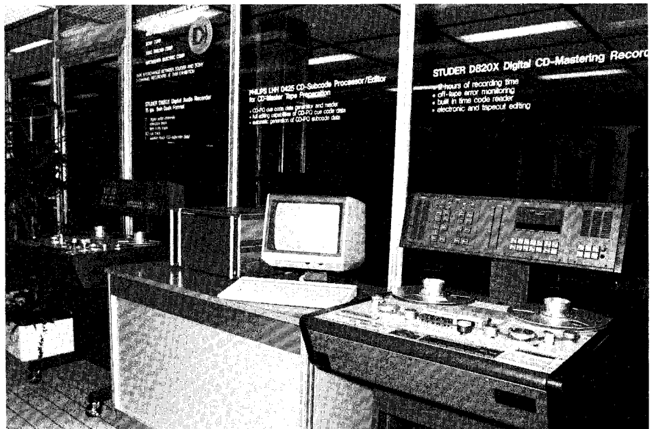
Digital audio engineering – Studer publicly demonstrated for the first time the compatibility of PCM machines in the twin DASH format. A Studer D820 X with a system for producing CD master tapes with subcode data was in action at the same time.
